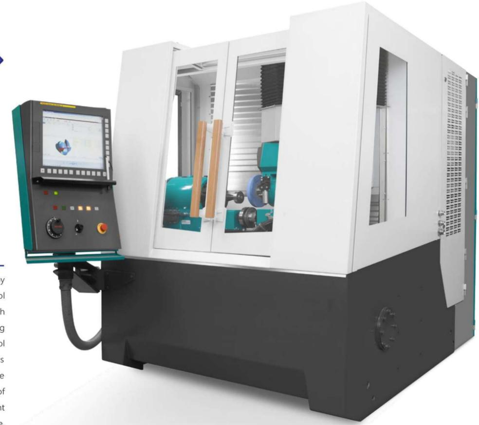
The machine is manufactured by Swiss Schlierberg machine Tool Manufacturing Company, which has 115 years of manufacturing history of high-precision tool grinders for various types of gear shaper grinding. The precision dimension stability of this equipment is very excellent in the grinding of cutter profile, and the profile size can meet the DIN AA grade standard.
